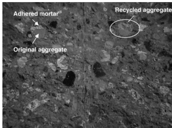
Fig. 2: Recycled aggregates concrete failure way by tensile ( M. Etxeberria et al, 2007 ).
