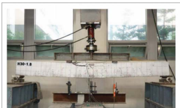
Fig.3: Beam testing for flexure (Thomas H.K. Kang et al. 2014).
